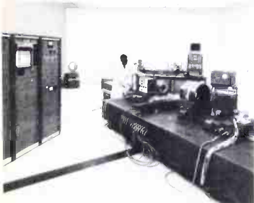
Eros IV Image Evaluator System of Ealing Corp. used by Perkin-Elmer Corp. to test MTF for ABC.
